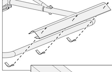
Place the clamp around the front tube and position the clamp so it hooks into the wind deflector.
